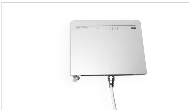
Fig. 12: Connect the LAN cable to the router
