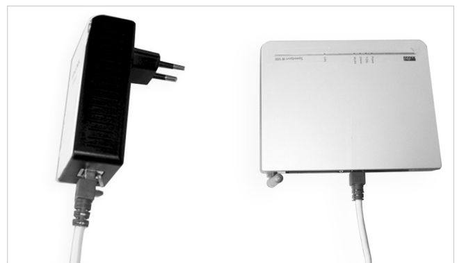
Fig. 14: Connecting a power line adapter to the router
